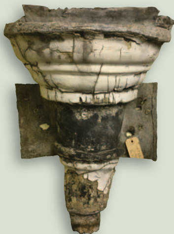
Late 18th century tapering semi-circular design, c.1780–89. The lead flaps that originally covered the wrought-iron fixings have been lost.
