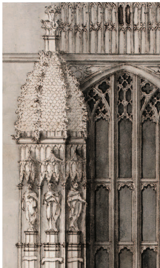
Fig. 20. Detail of Dickinson's drawing of the crocketed cone of the polygonal turrets of the Henry VII chapel, black and brown ink and grey wash over pencil, no date. ( WAM(P) 913A. © Dean and Chapter of Westminster )
