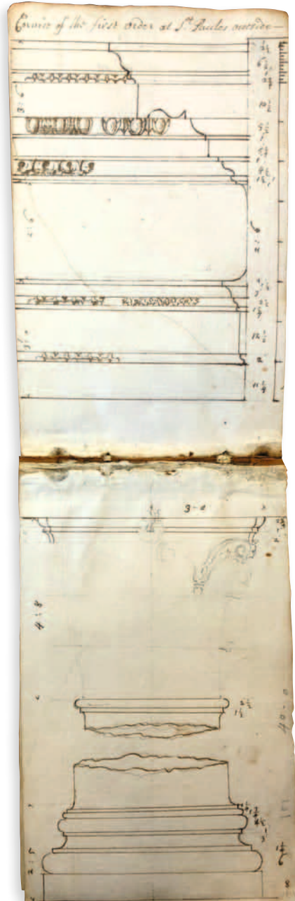
Fig. 2. Dickinson's measured drawing for the 'Cornice of the first order at St Pauls outside' of the dome, black ink over pencil, c.1701-2. ( MS Gough Misc. Antiq. 17, f. 100r-101v © Bodleian Libraries, University of Oxford)
